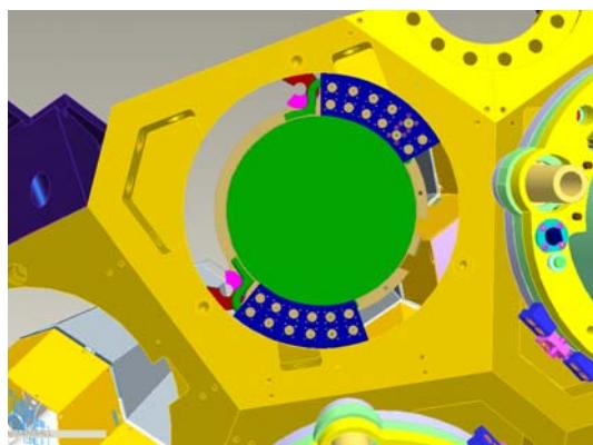
Image on the left showing the cryostat a tight fit when installed, mounting ring has to be replaced, probably connector brackets need to be repositioned /redesigned.
