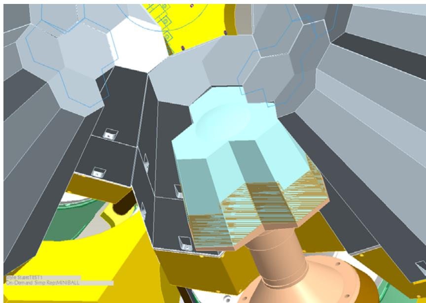
Above image shows Miniball detector beside Agata triples. Two triples withdrawn, 1 miniball inserted. Surprising close fit, although a slight clash at 235 radius. It comes clear at 232 radius, if brought back by itself, If all the AGATA detectors are brought back together this would allow a radius of approx 233.
