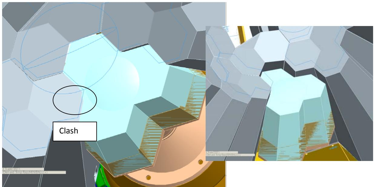
Miniball clashes with AGATA detector. Miniball Detector has be withdrawn aprox 20mm to come clear. AGATA detectors remain at 235.
